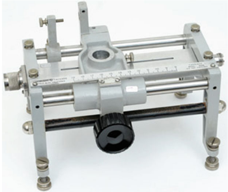
Fig. 7.3 Waveguide slotted line carriage
